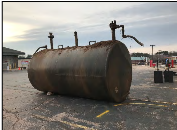
4,000 gallon leaded (race gas) UST
