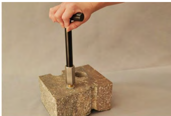
Figure 7. Removing the Vapor Pin™.
