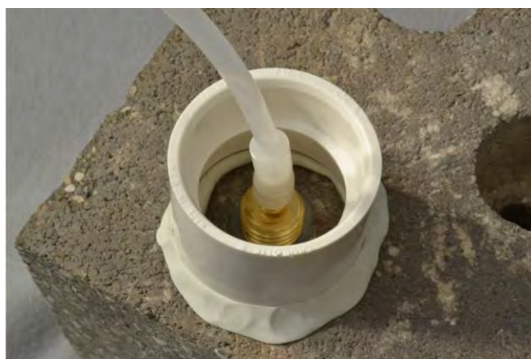
Figure 6. Water dam used for leak detection
