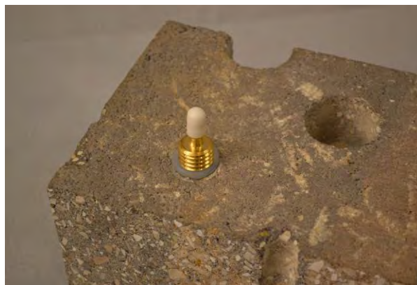
Figure 3. Installed Vapor Pin™
