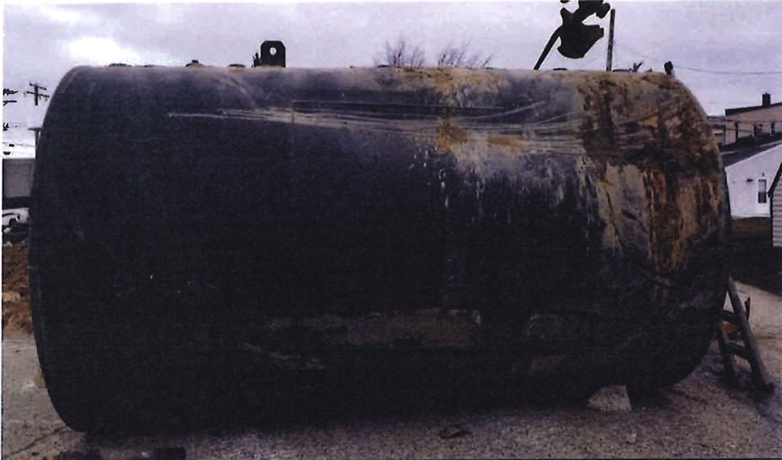
PHOTO 1 – PHOTOGRAPH OF 6,000-GALLON UST FROM SOUTHERN TANK EXCAVATION
