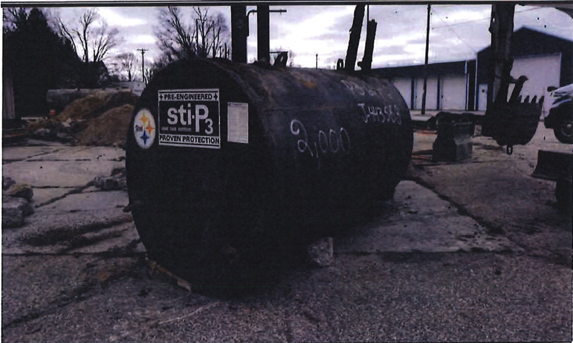
PHOTO 7 – PHOTOGRAPH OF THE 2,000-GALLON DIESEL UST FROM THE NORTHERN EXCAVATION
