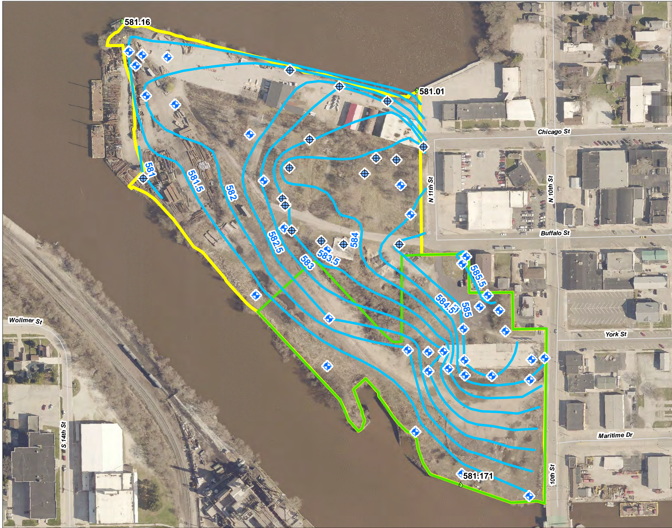
Figure No. 6 Title Groundwater Elevation at the River Point District (March 2021) Client/Project Site Investigation Project Area River Point District City of Manitowoc 0 125 250 Feet Prepared by HLB on 4/21/21
