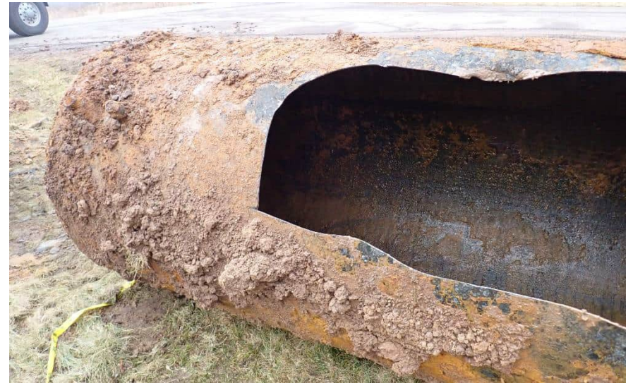
Interior of removed 750-gallon tank.
