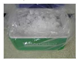
D. Place large bag of ice or loose ice on top of the bottles. In warm weather, the cooler should be packed with as much ice as possible.
