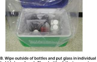
B. Wipe outside of bottles and put glass in individual bubble bags & seal. Place bottles & the temperature blank into cooler. Leave room for ice in between bottles & on top.
