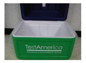
A. Line cooler with bubble wrap and large plastic bag. Use absorbent pad inside the bag if bottles contain preservatives.
