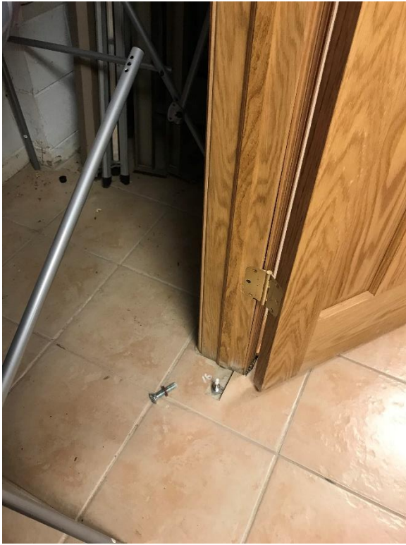
Photo 13: RA Environmental sub-slab vacuum observation point fitted with vapor pin for sub-slab pressure field extension testing, typical 08/06/2019
