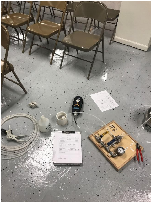
Photo 19: Sub-slab vapor sampling equipment at sub-slab depressurization mitigation system cleanout sample location, typical 08/14/2019
