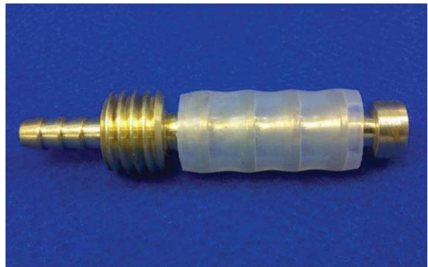
Figure 1. Assembled VAPOR PIN®
