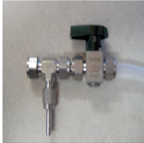
Photograph 17 - T-connection for quantitative tracer gas
