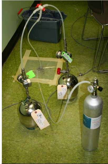
Photograph 15 - Field duplicate sample collection setup
