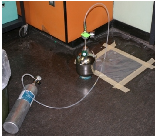
Photograph 21 - Plastic wrap leak detection method during sampling
