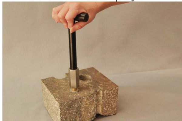
Figure 7. Removing the VAPOR PIN®
