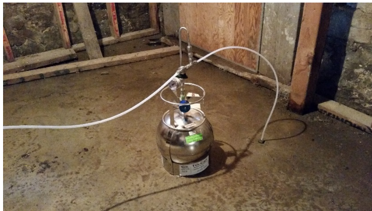
Photograph 6 – Sample collection at temporary sub-slab vapor point
