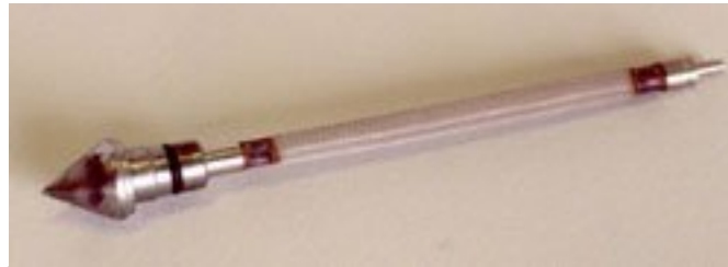
Photograph 7 – Stainless-steel mesh soil vapor point
