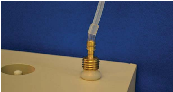
Figure 5. VAPOR PIN® sample connection
