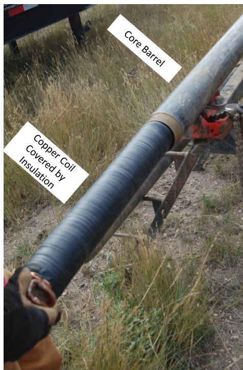
Figure S-2. Insulated cooling coil being inserted into the core barrel.
