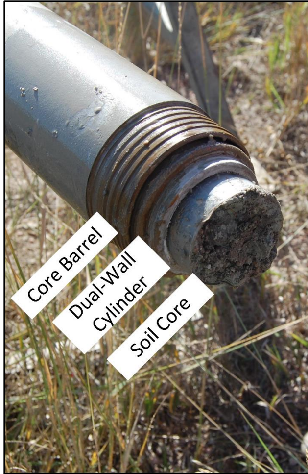
Figure S-3. Dual-wall cooling cylinder inserted into the core barrel.
