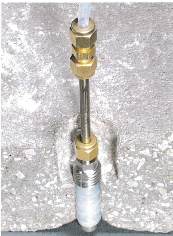
Figure 7. FLX-VP™ with TO-17 Sorbent tube connection
