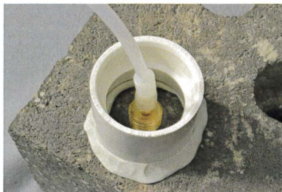
Figure 8. Water dam used for leak detection
