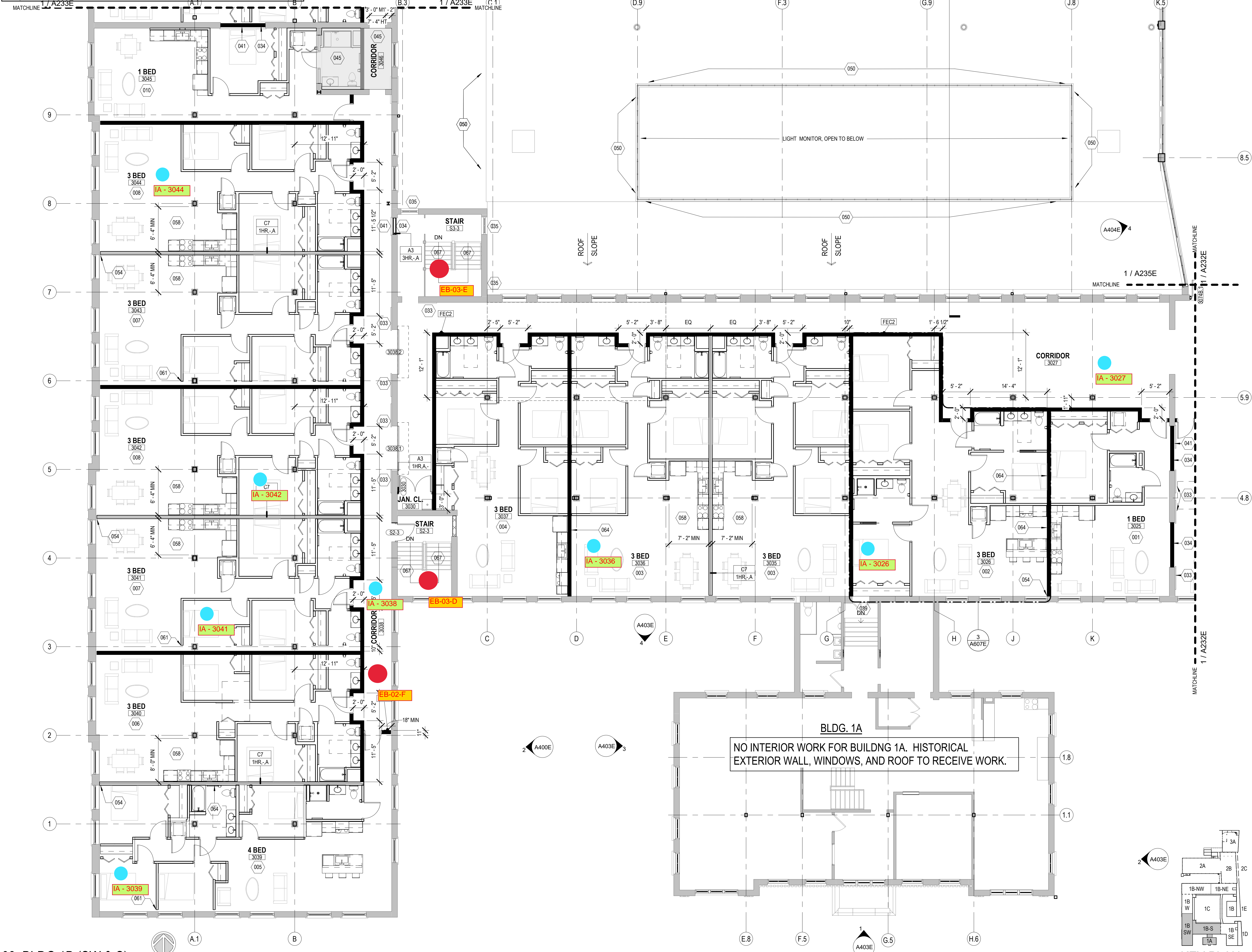
1 NEW WORK PLAN - LEVEL 02, BLDG 1A & LEVEL 03, BLDG 1B (SW & S) Scale: 1/8" = 1'-0"
