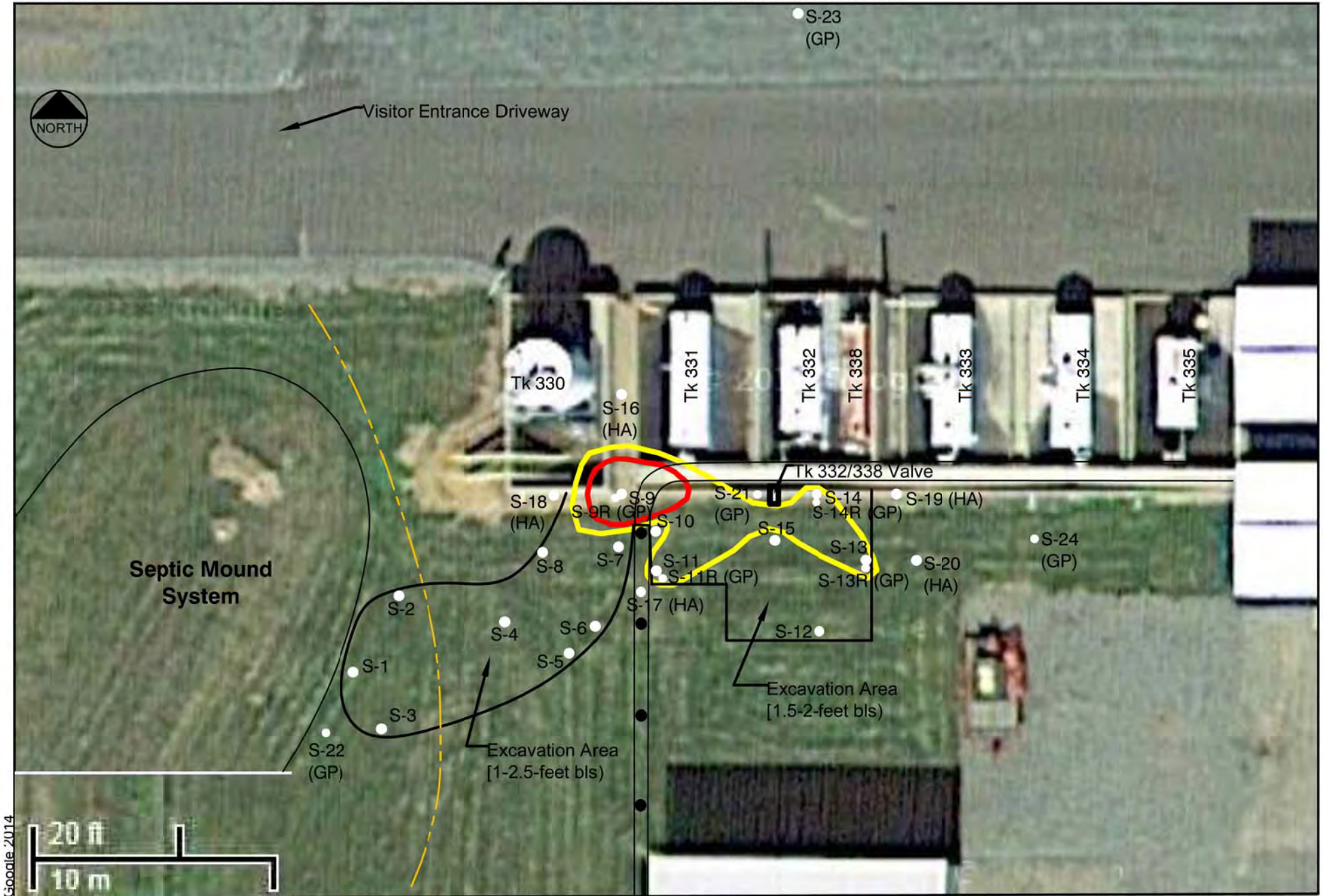
Figure B.2.a Soil Contamination Additive Tk 338 Release FHR Pine Bend, LLC Fuel Terminal 2267 County Highway HH, Junction City, WI
