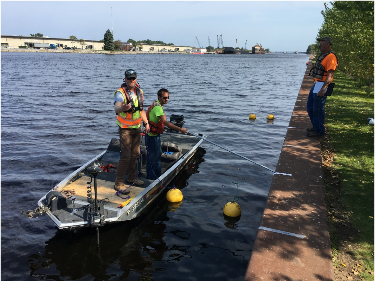
Figure 2. Deployment of SCUFA Moorings at T3 with Two Moorings 25 feet Downstream of Injection and Two More 50 feet Downstream
