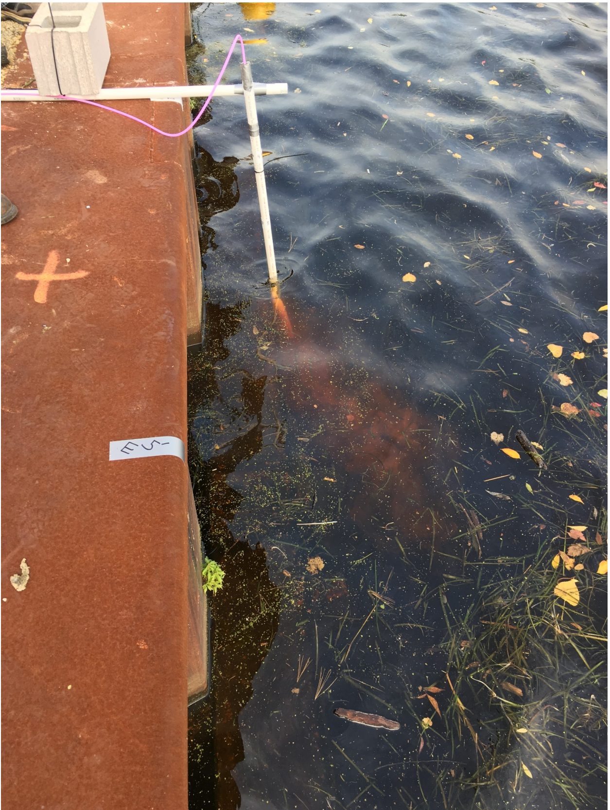
Figure 9. Dye Plume at Location T1 in Turning Basin with Visible Plume Moving East under Weak and Variable Currents. Tape Marks 5 Feet East of Injection Location, 2 Feet Below the Water Surface.
