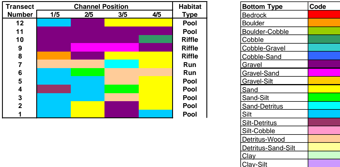
Figure 20. Bottom sediment map and key for the survey site upstream of Highway T on Logan Creek. Transect 1 is the furthest downstream sampling location.
