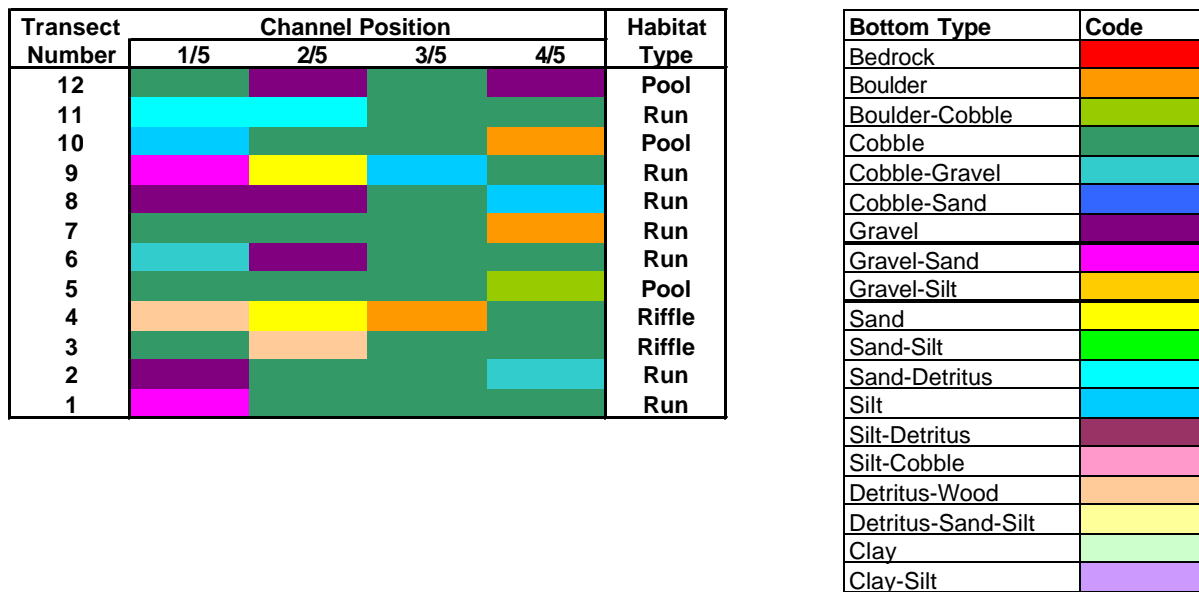
Figure 33. Bottom sediment map and key for the survey site upstream of Gardner Road on Sugar Creek. Transect 1 is the furthest downstream sampling location.
