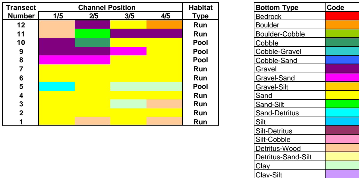
Figure 45. Bottom sediment map and key for the survey site upstream of County U on Woodward Creek. Transect 1 is the furthest downstream sampling location.
