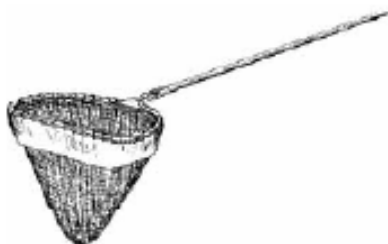
Figure 5-3. D-frame net used for collecting benthic macroinvertebrates.
