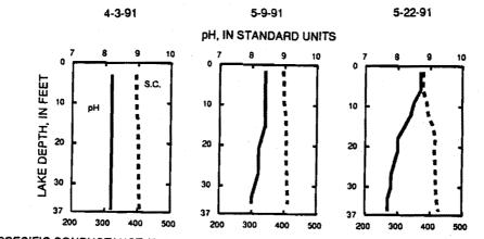
SPECIFIC CONDUCTANCE (S.C.), IN MICROSIEMENS PER CENTIMETER AT 25 DEGREES CELSIUS
