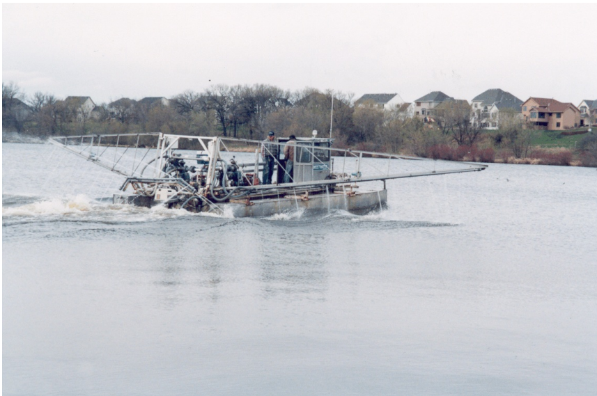
Figure 34. An alum application is generally applied from a barge. This was a lake sediment alum application on Lake Susan in Chanhasen.
