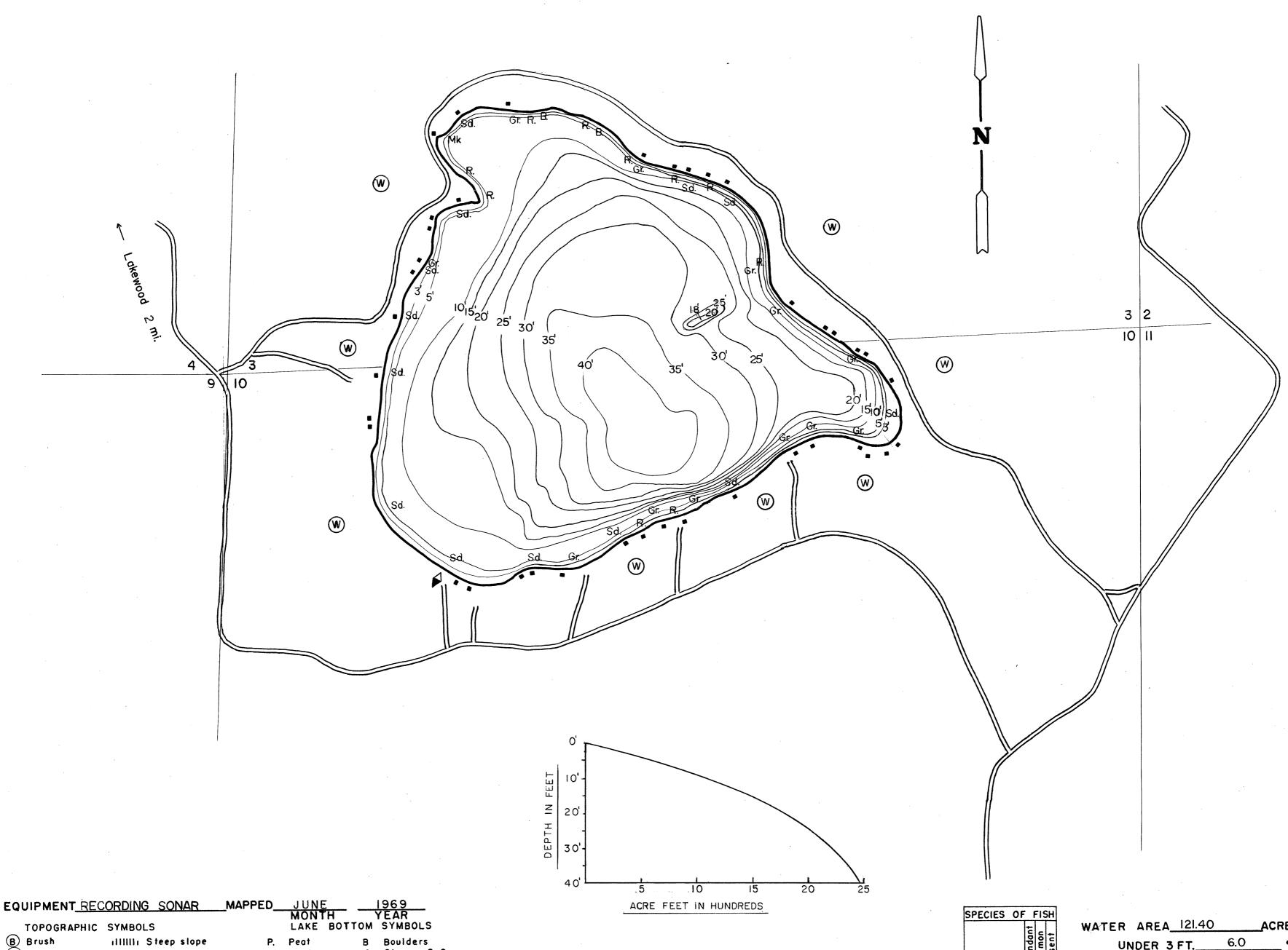
TOPOGRAPHIC SYMBOLS B Brush % Stumps & Snags Mk. Muck C. Clay Rock danger to navigation Submergent vegetation M. Mari P Pastured \_\_\_\_\_Intermittent stream Sd. Sand Emergent vegetation (A) Agricultural \_\_ Floating vegetation St. Silt Permanent inlet Permanent outlet → Brush shelters Gr. Gravel B.M. Bench Mork **↓** Dam R. Rubble ■ Dwelling Resort
