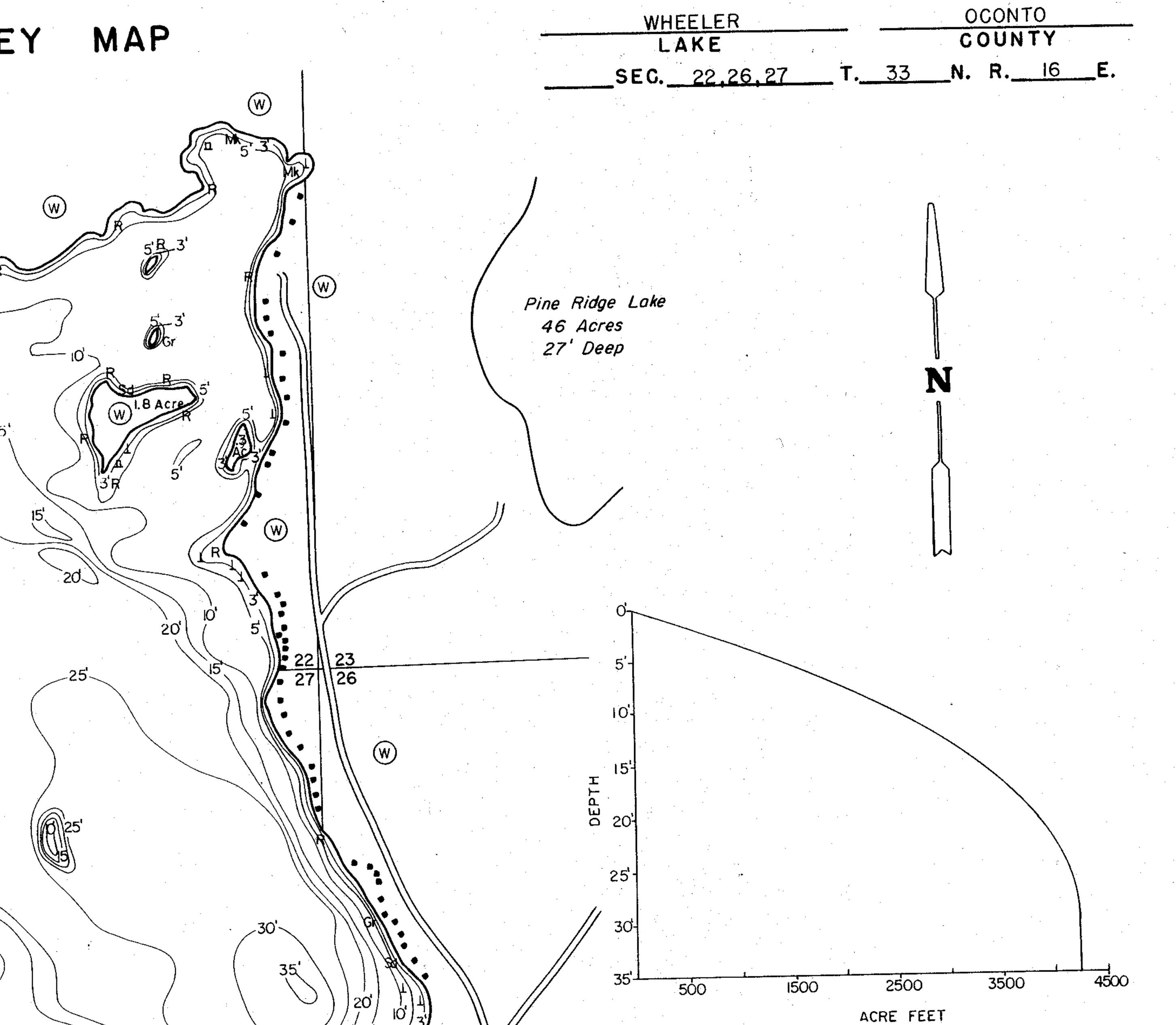
B.M. 'X' D.N.R. 1741-C 2" square cut in N.W. corner of concrete base of water pump 57.6' S.W. of B.M. 'X' 1741-B, 52' S. of lake Assumed elevation 100.93' Water level 98.23'
