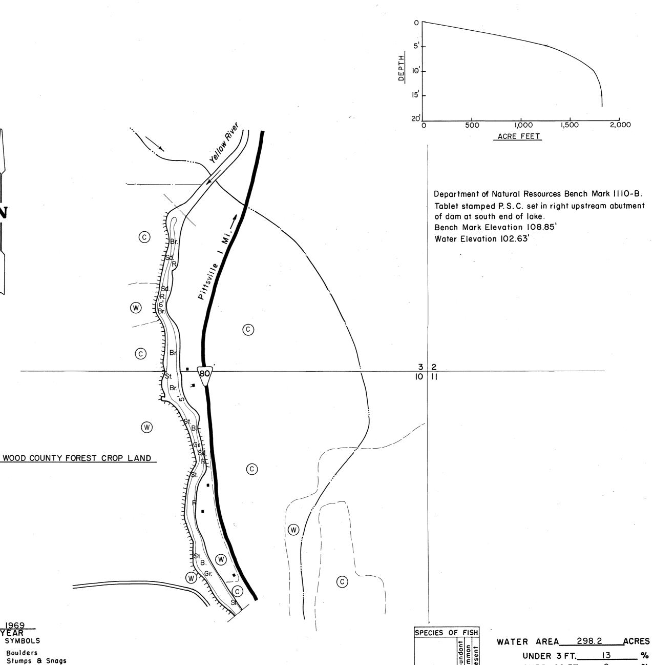
EQUIPMENT RECORDING SONAR MAPPED\_ LAKE BOTTOM SYMBOLS TOPOGRAPHIC SYMBOLS B Brush illilli Steep slope P. Peat Boulders Stumps & Snags Mk. Muck C. Clay Rock danger to navigation M. Marl Submergent vegetation Sd. Sand 1 Emergent vegetation \_\_\_\_ Intermittent stream A Agricultural St. Silt \_ Floating vegetation Permanent inlet Brush shelters B.M. Bench Mark Permanent outlet Gr. Gravel
