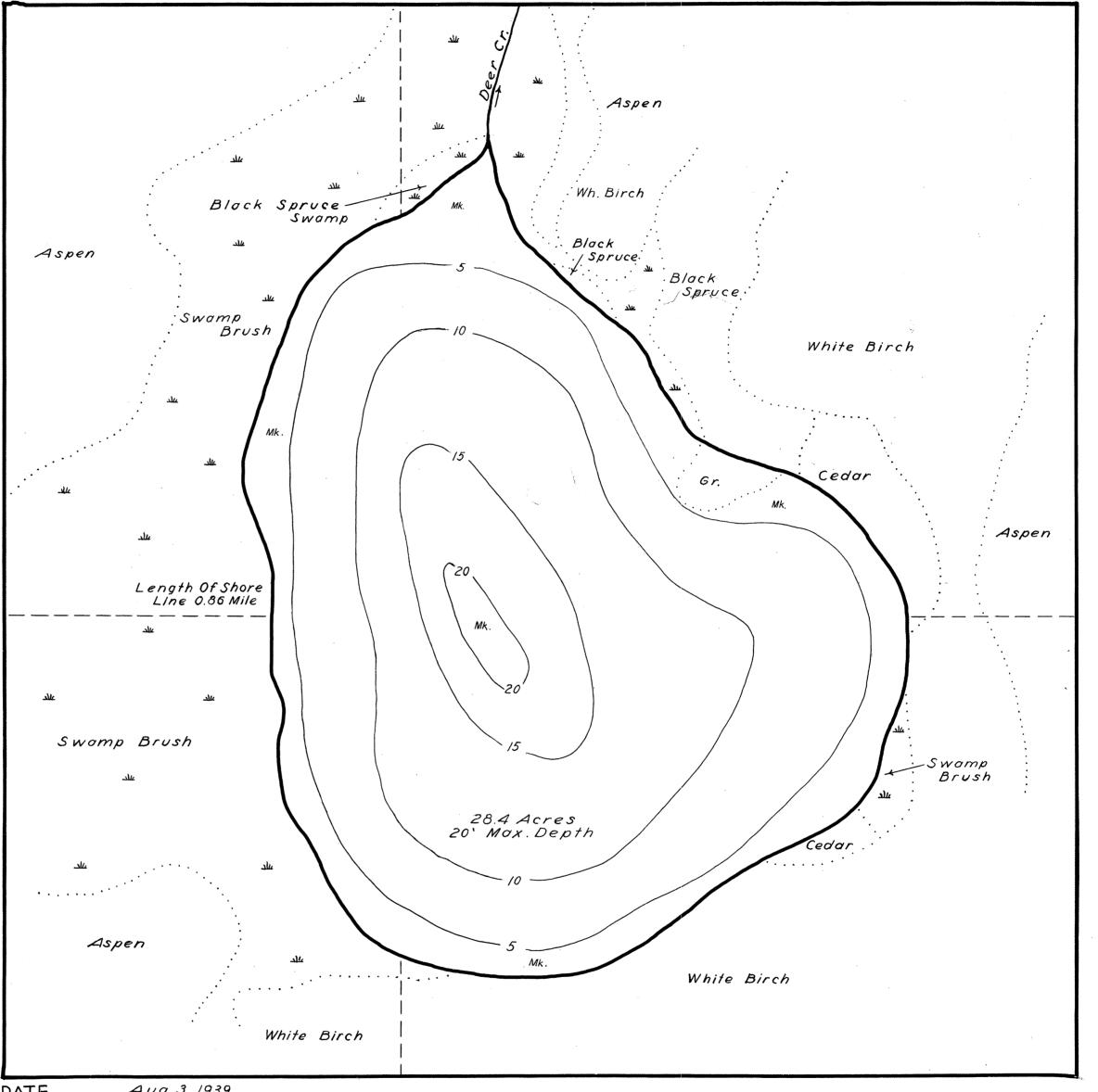
Aug. 3. 1939 DATE\_ SCALE | linch = 165 feet COMPILED BY\_ TRACED BY\_ R.F.F (W.P.A) LAKE IMPROVEMENT RECORD SOURCE OF INFORMATION TYPE DATE \_\_ LEGEND U.S. Forest Service Lake And OBRUSH REFUGES\_\_\_\_\_ ₩EED BEDS Stream Survey - SAPLING TANGLES ☐ SPAWNING BOXES\_\_\_ \*\* MINNOW SPAWNERS. SOUNDINGS At 5' Intervals Sd SAND U.S. Forest Service C. CLAY Gr. GRAVEL TOTAL DATES OF MAP REVISION\_ Mk MUCK ■ DWELLING □ ABANDONED DWELLING WORK AGENCY\_ **■** RESORT
