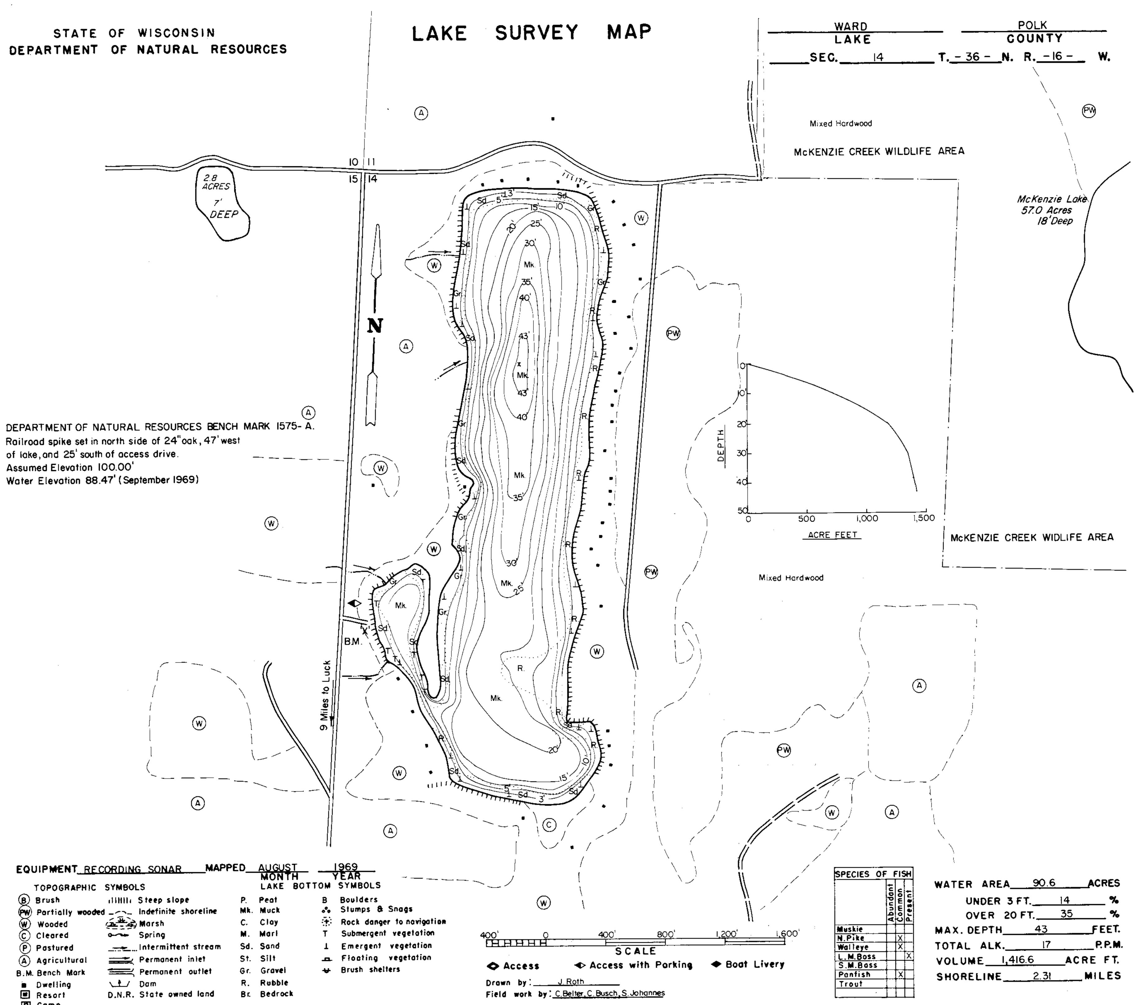
Railroad spike set in north side of 24"oak, 47'west of lake, and 25' south of access drive. Assumed Elevation 100.00<sup>4</sup> Water Elevation 88.47 (September 1969)
