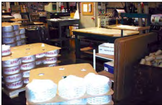
Printpack uses rolls of plastic film to produce “flexible packaging” for candy bars and other products; it recycles the scrap film. Photo courtesy Printpack Inc.
