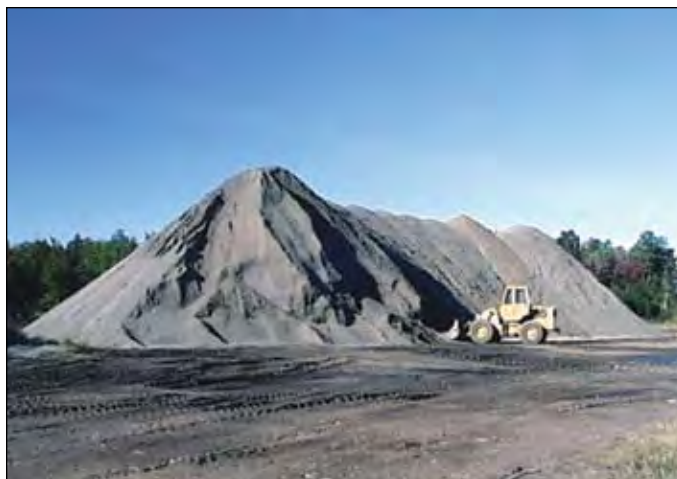
A pile of crushed concrete being recycled by PCA’s Tomahawk plant. The concrete is used in construction projects such as a new parking pad for semi trucks. Photo courtesy PCA.
