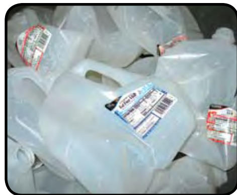
N.E.W. Plastics Corp. of Luxemburg uses plastic from milk jugs (bottom) and other containers to manufacture plastic sheeting for truck liners (top) and plastic lumber. (Top photo by Robert Queen; bottom photo by Karin Olefsky.)
