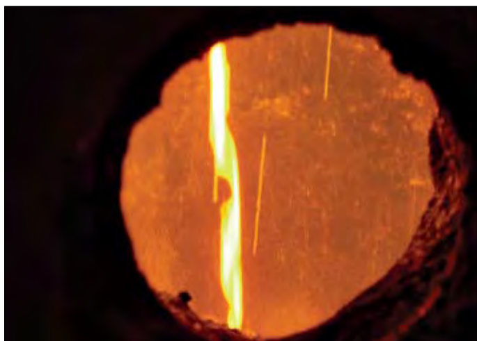
Molten glass exits a cyclone furnace at Minergy's Fox Valley Glass Aggregate Plant. Photo courtesy Minergy Corp.
