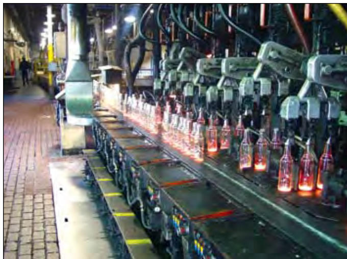
Glass bottles are manufactured and filled at the Saint-Gobain plant in Burlington. Recycled glass is incorporated into the containers. Photo courtesy Saint-Gobain Containers.
