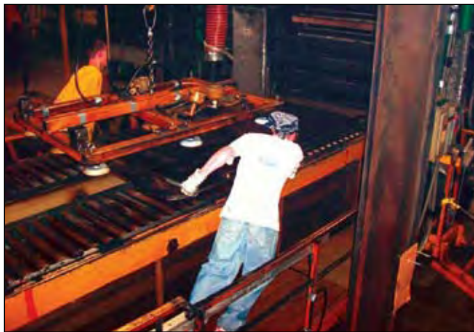
Workers push a full mold into a press at Humane Manufacturing’s Janesville plant. Photo courtesy Humane Manufacturing Company LLC.
