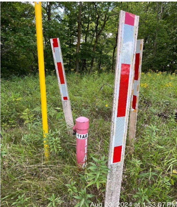
Photo 6: Ring of brightly colored posts around a groundwater monitoring well.
