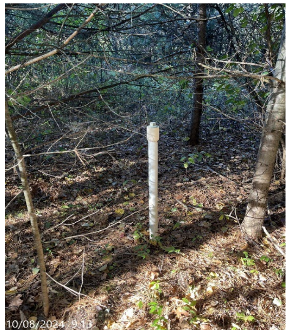
Photo 4: Groundwater monitoring well casing without protective cover pipe or lock.
