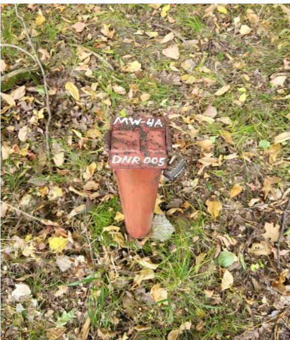
Photo 8: Well label written on the protective cover pipe clearly showing the well name and GEMS point ID.
