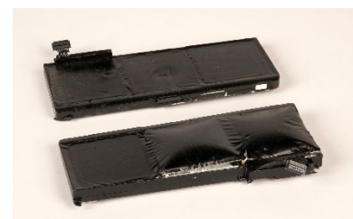
Comparison of normal and damaged lithium-ion batteries
