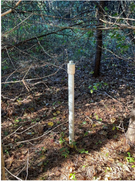
Photo 18: Groundwater monitoring well that needs a metal outer protective casing installed.
