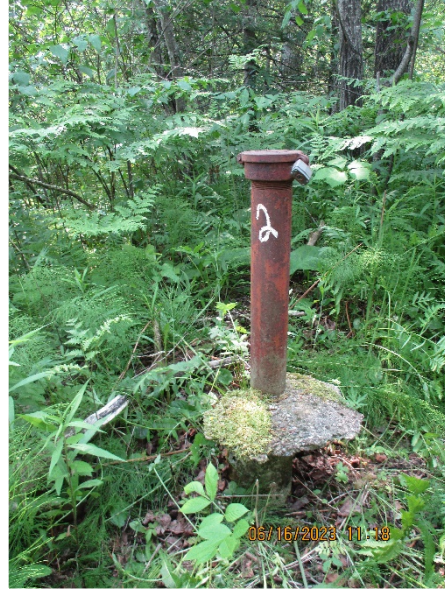
Photo 19: Groundwater monitoring well with concrete surface seal that has heaved out of the ground due to frost.
