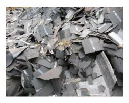
Residential asphalt shingles (RAS) are easy to identify in both roofing tear-off waste and in general construction and demolition (C&D) waste. The licensing requirements for various RAS handling activities may not be as easily identified.
