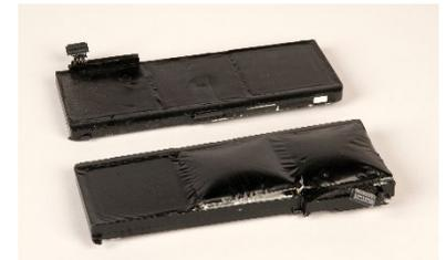
*Comparison of normal and damaged lithium-ion batteries*
