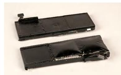
*Comparison of normal and damaged lithium-ion batteries*
