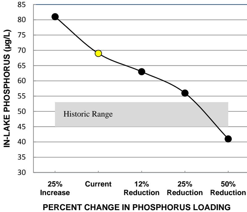
Figure 11 – Response of Poskin Lake to Phosphorus Loading Reductions
