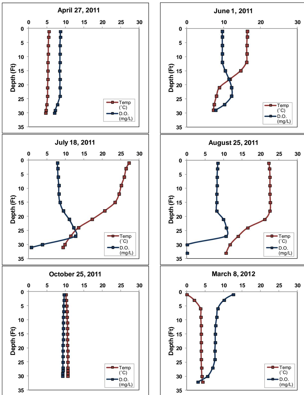
Figure 3.1-7. Lake Mildred dissolved oxygen and temperature profiles. The March 8, 2012 profile was collected through the ice.
