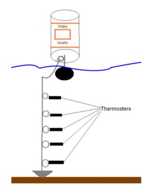
Figure 24. Diagram depicting how the thermistors were deployed at BL02 (diagram is not to scale).
