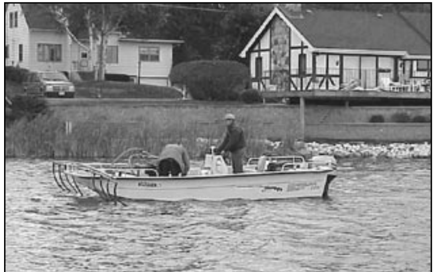
Fluridone is typically applied through subsurface injection with hoses that drag in the water.
