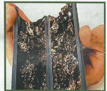
zebra mussels in a intake pipe (Photo from Michigan Sea Grant Archives)
