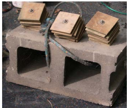
Figure 1. Three Hester-Dendy samplers attached to cinder blocks.
