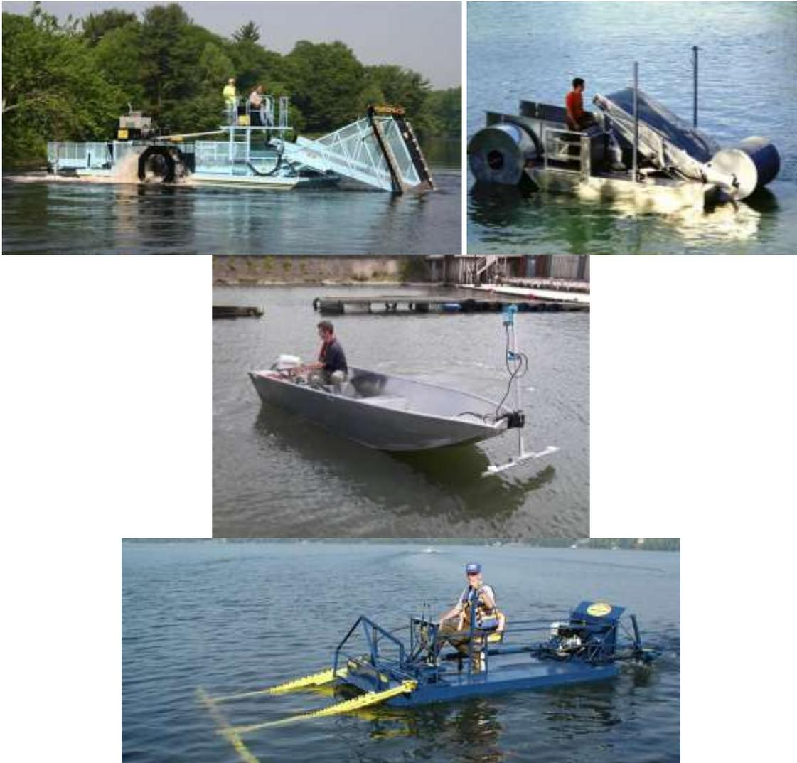
**Figure 12: Examples of different size and type of aquatic plant harvesters (Aquarius Systems, Eco-Harvester, Jenson Lake Mower, Hockney Weed Cutter)**
