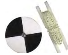
Figure 3: A Secchi disc, which is lowered into the water to measure water clarity
