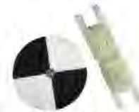
A Secchi disc, which is lowered into the water to measure water clarity
