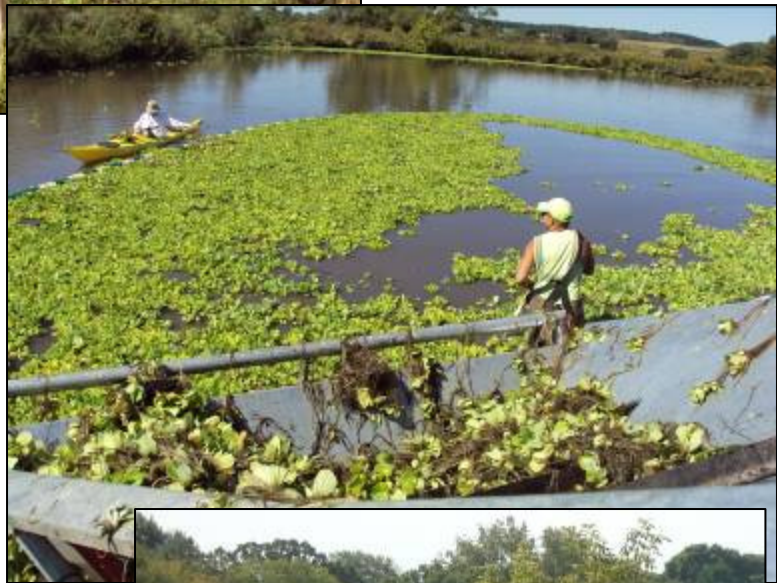
Workers slowly pull the boom as the kayakers pushed against the boom to corral the plants towards the conveyer belt in calm winds.
