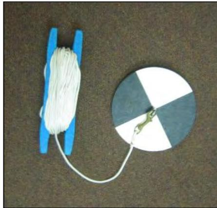
**Figure 15. A secchi disk, a tool used to measure water clarity.**
