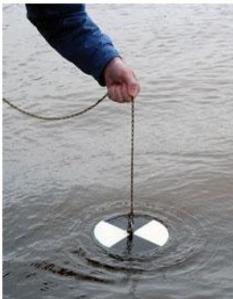
**Figure 22: Photo of Testing Water Clarity with Secchi Disk**
