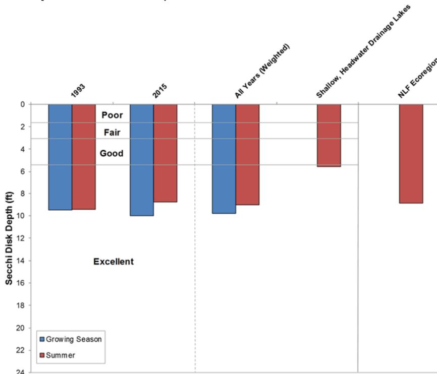
**Figure 8.1.1-3. Pickerel Lake, state-wide shallow, headwater drainage lakes, and regional Secchi disk clarity values.** Mean values calculated with summer month surface sample data. Water Quality Index values adapted from WDNR 2012A.
