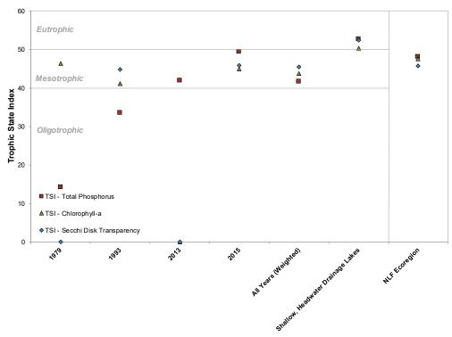
**Figure 8.1.1-4.** Pickerel Lake, state-wide shallow, headwater drainage lakes, and regional Wisconsin Trophic State Index values. Values calculated with summer month surface sample data using WDNR 2012A.
