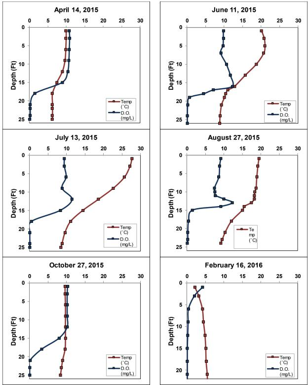
Figure 8.2.1-6. Little Pickerel Lake dissolved oxygen and temperature profiles.
