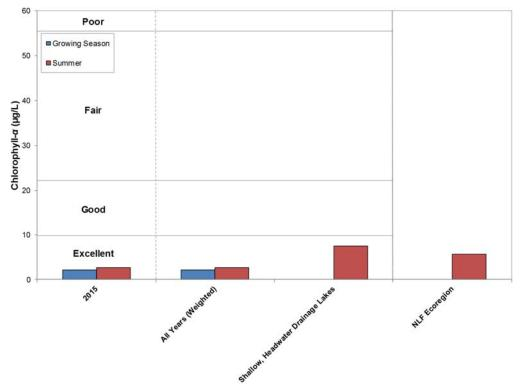
**Figure 8.3.1-2.** Smoke, state-wide shallow, headwater drainage lakes, and regional chlorophyll-a concentrations. Mean values calculated with summer month surface sample data. Water Quality Index values adapted from WDNR 2012A.
