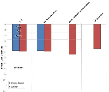
**Figure 8.2.1-3.** Little Pickerel Lake, state-wide deep, headwater drainage lakes, and regional Secchi disk clarity values. Mean values calculated with summer month surface sample data. Water Quality Index values adapted from WDNR 2012A.
