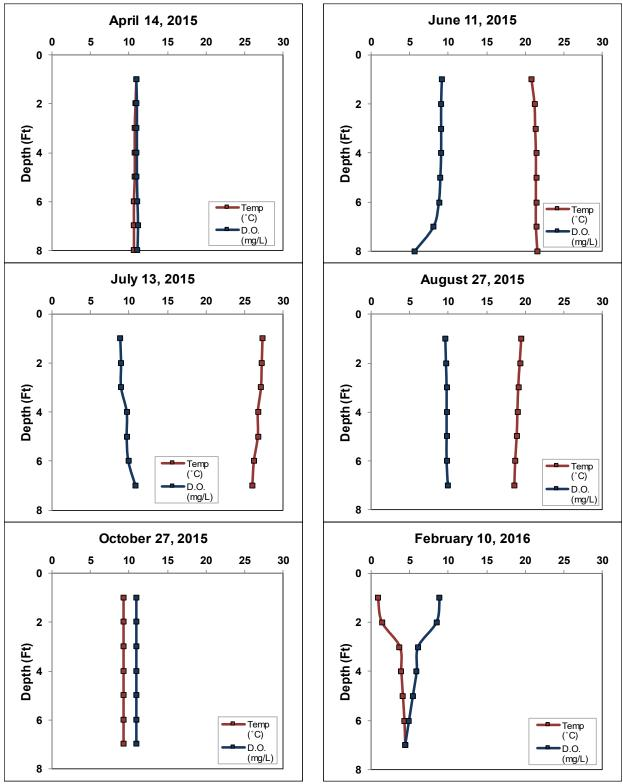
Figure 8.3.1-4. Smoke Lake dissolved oxygen and temperature profiles.
