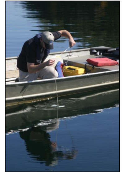
A secchi depth measure being taken on a lake. Photo by Laura Herman.
