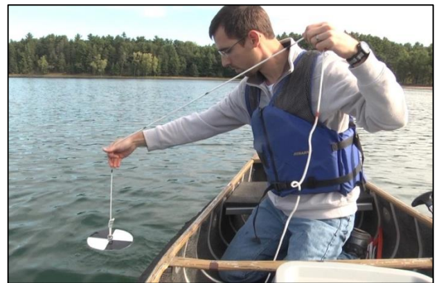
Secchi disk reading being taken on Sunset Lake. Photo by Amy Kowalski.
