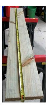
4. A third hole for the lag bolt needs to be marked off at 45 inches (1.5 inches above the bottom marking). This will be used by the surveyors to anchor the stadia rod.
