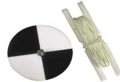
A Secchi disc, which is lowered into the water to measure water clarity
