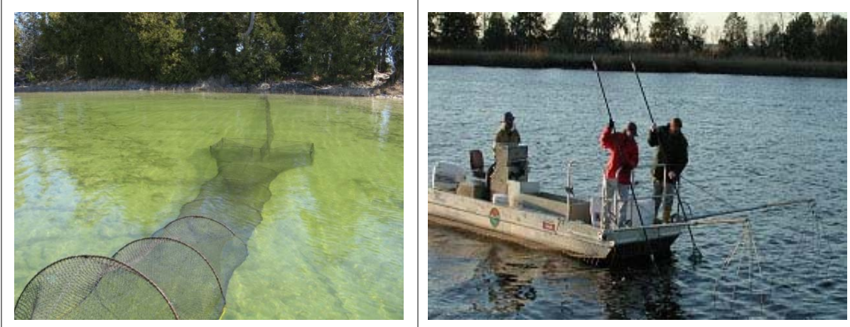
Photo 8.3.6-1. Fyke net positioned in the littoral zone of a Wisconsin lake (right) and an electroshocking boat (left).
