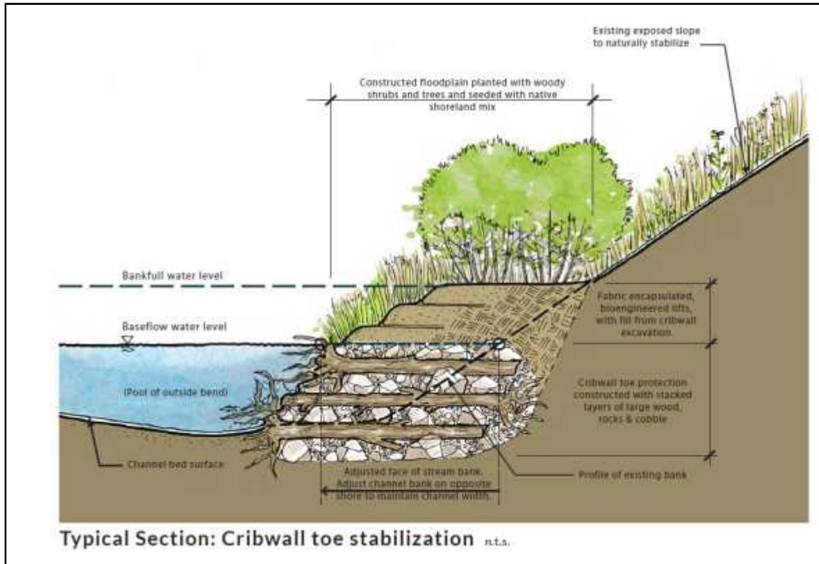
Figure 30. Schematic of a cross section through a log cribwall.
