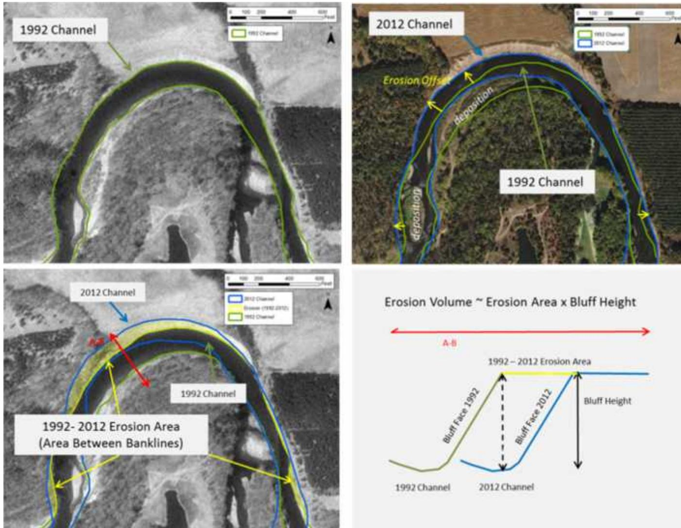
Appendix H. Estimation of Erosion Process. 1) Banklines were drawn along the channel on each photograph, and then compared. 2) Erosion areas were delineated as the area between banklines. 3) The maximum offset is the maximum distance between the two banklines, and the average offset is the average distance between the lines. 4) Erosion volumes were estimated by multiplying the erosion area by the height of the bank or bluff.
