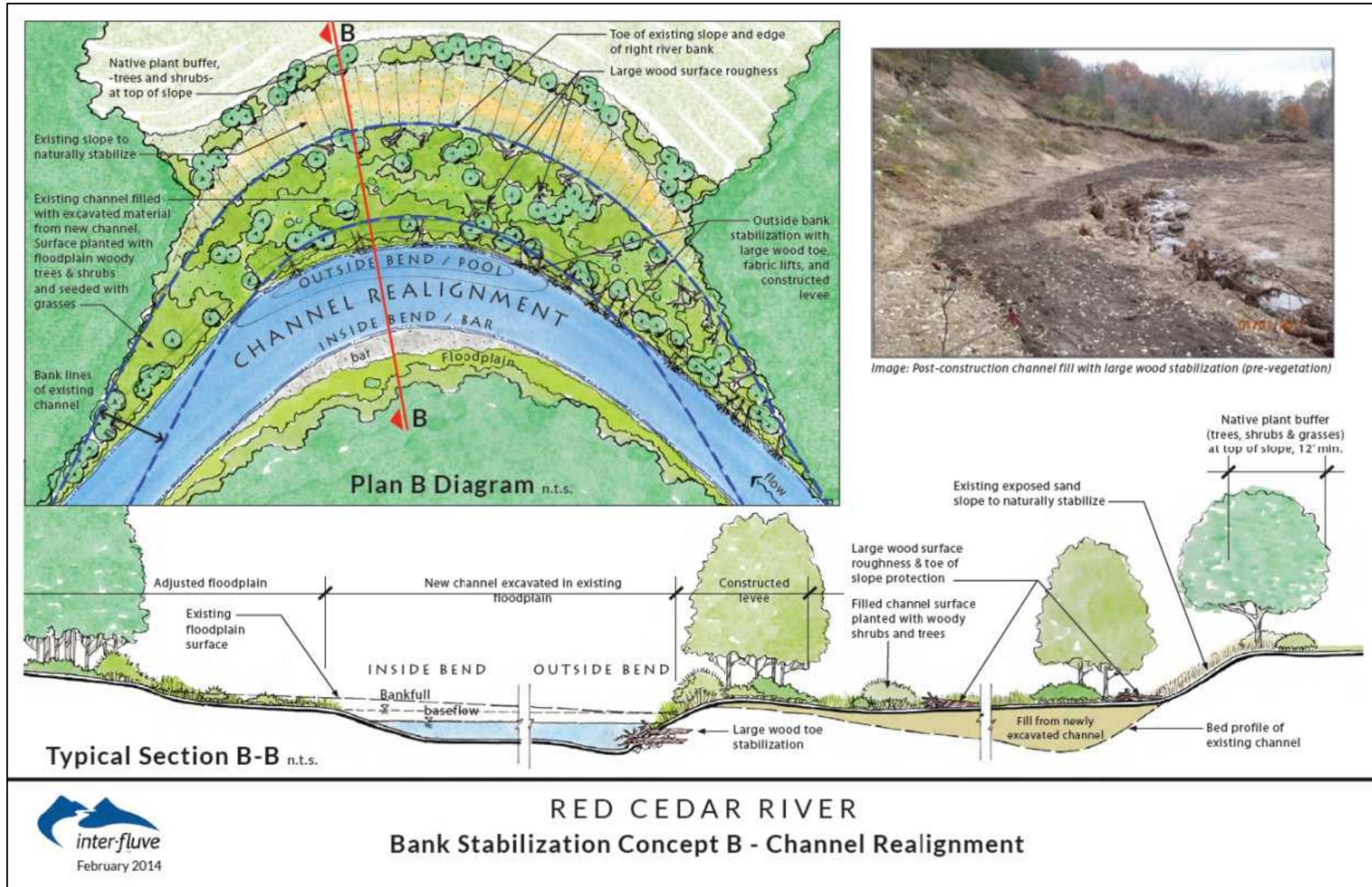
Appendix K. Planview schematic of a log cribwall stabilization project with a new channel constructed on the inside of the bend, and the existing channel filled and converted to floodplain.
