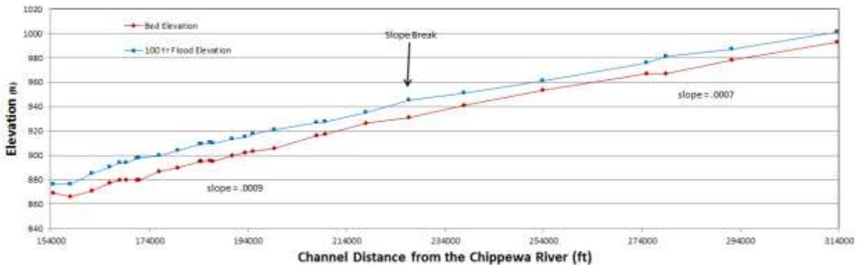
Figure 11. Long Profile of the Red Cedar River through Dunn County, WI. “Flood Elevation” represents the statistical 100 year return interval flood (from Dunn County Flood Insurance Study, FEMA 2008).
