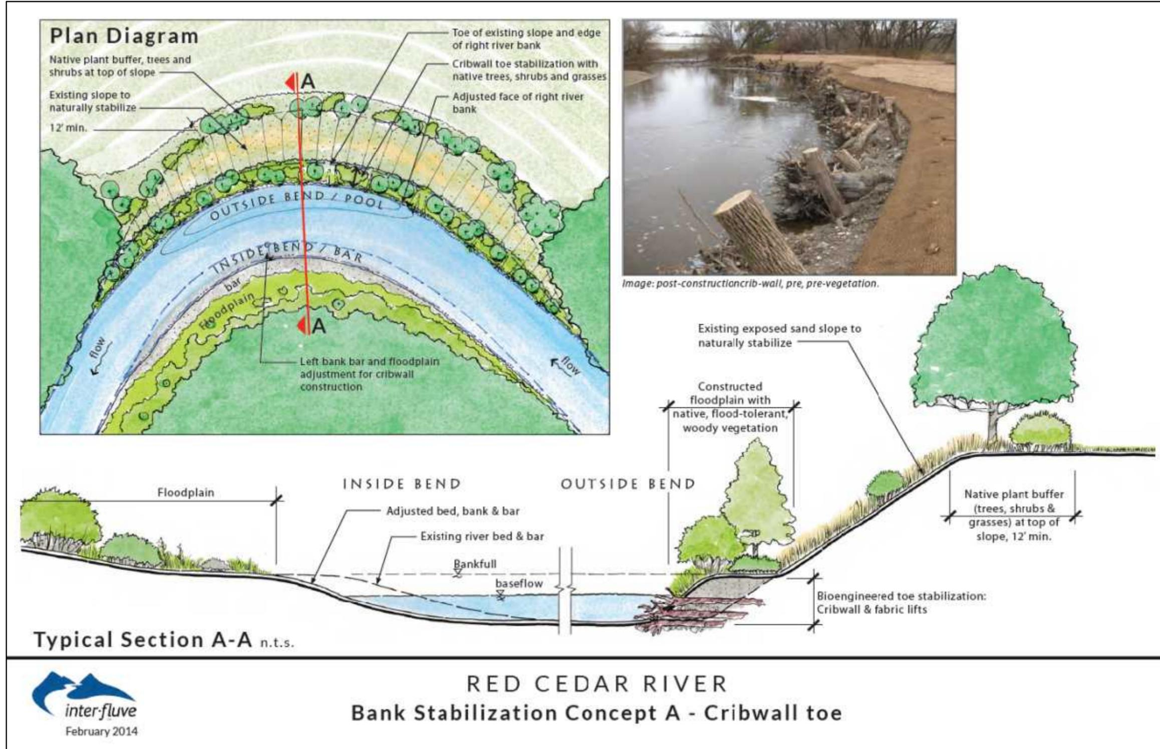
Appendix J. Planview schematic of a log cribwall stabilization project.
