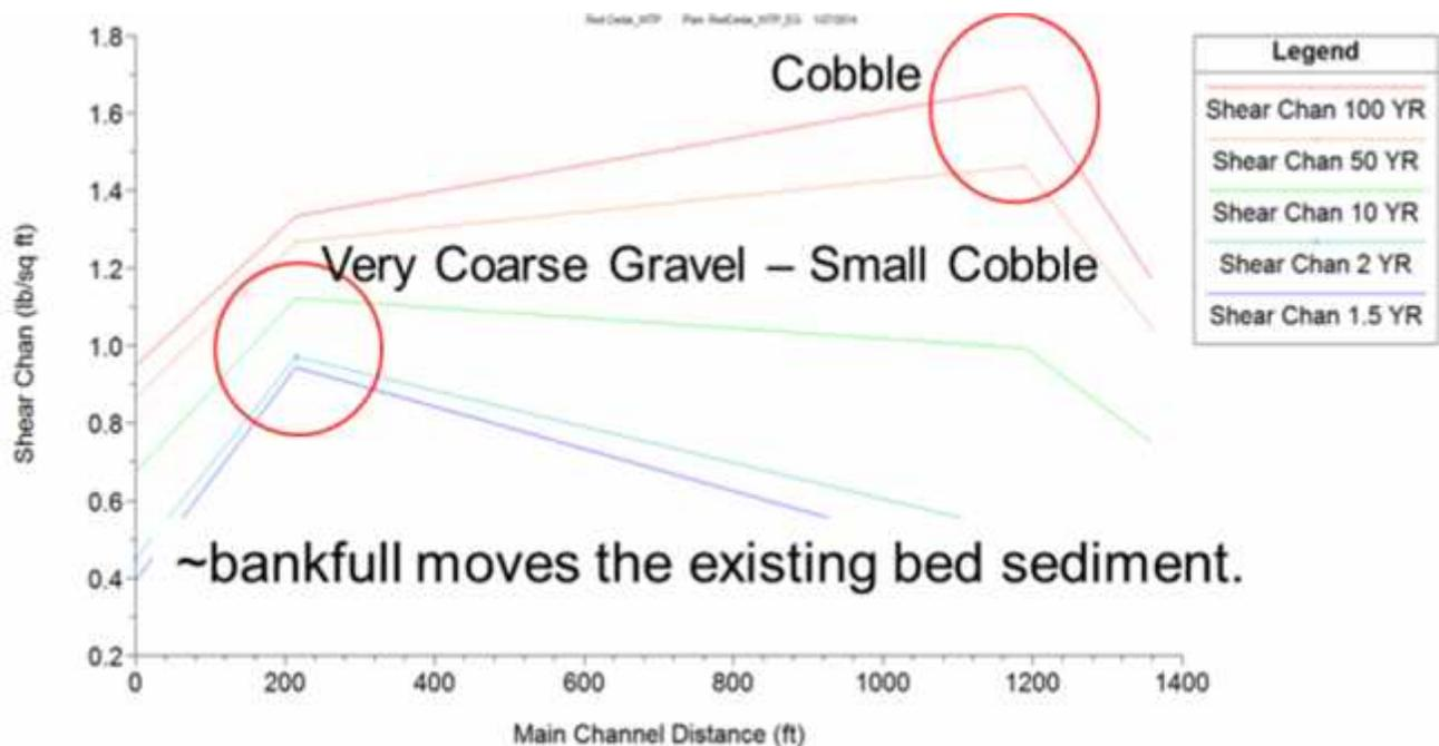
Figure 6. Shear stress results from HEC RAS model. At floods with recurrence intervals of at least 5 years, the shear stresses are large enough to mobilize coarse gravels. Extreme floods can move larger cobbles.
