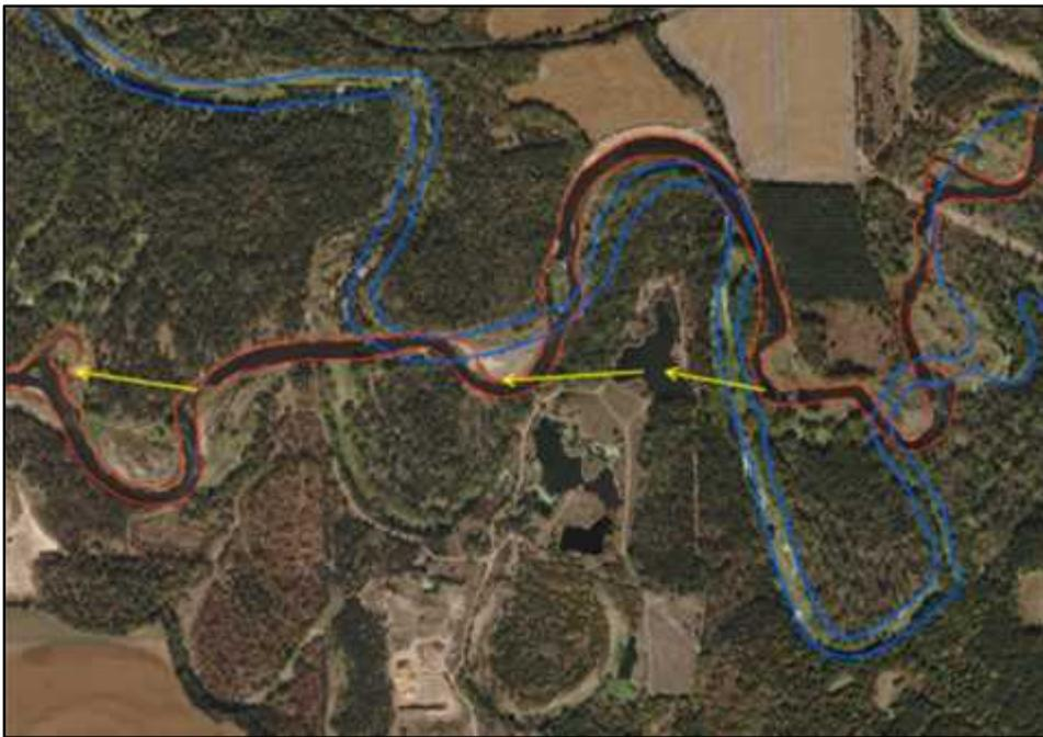
**Figure 35. Potential avulsion/chute cutoff path along the existing channel. The gravel pits on the south side of the channel provide preferential pathways for floodwaters to cut a new position.**
