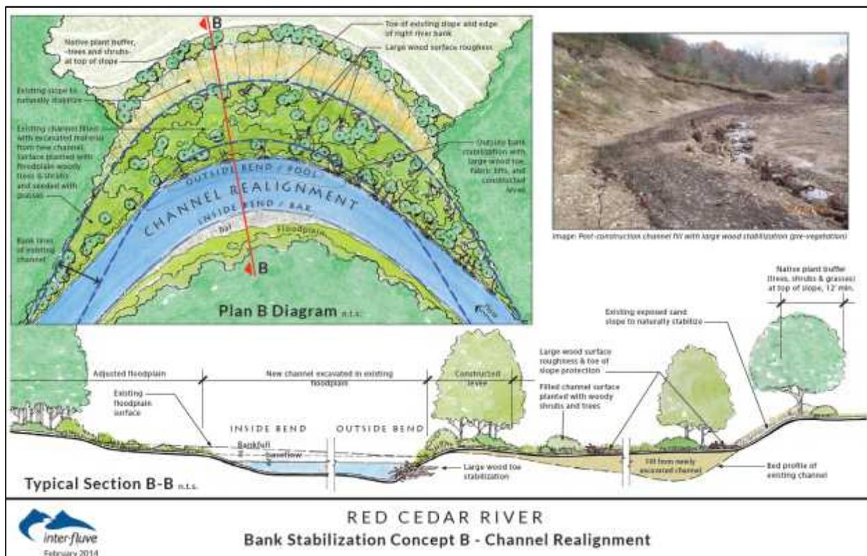
Figure 25. Planview schematic of a log cribwall stabilization project with a new channel constructed on the inside of the bend, and the existing channel filled and converted to floodplain.
