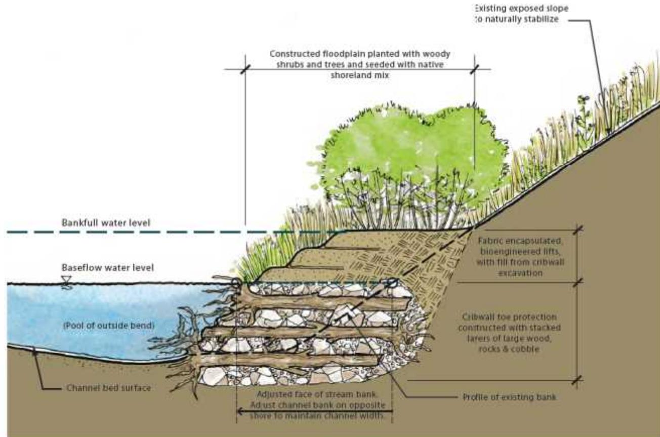
Typical Section: Cribwall toe stabilization n.t.s.
