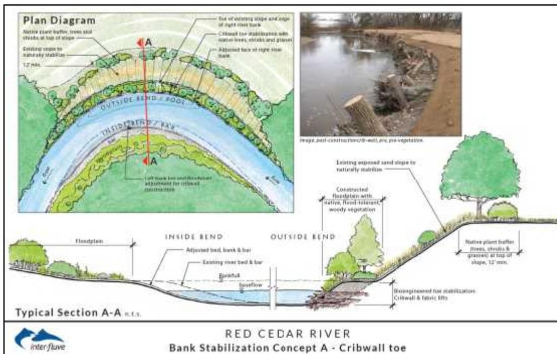
Figure 31. Planview schematic of a log cribwall stabilization project.
