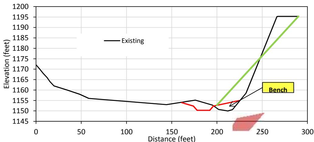
**Figure 24. Existing, proposed and expected typical cross section at a typical bluff stabilization site. The existing ground (black line) shows the channel scouring at the toe of the bluff on the right side of the valley. The proposed channel (red line) will be excavated away from the bluff toe to allow room for placement of the treatment (riprap or cribwall) and to provide room for the upper bank material to slump over (green line).**
