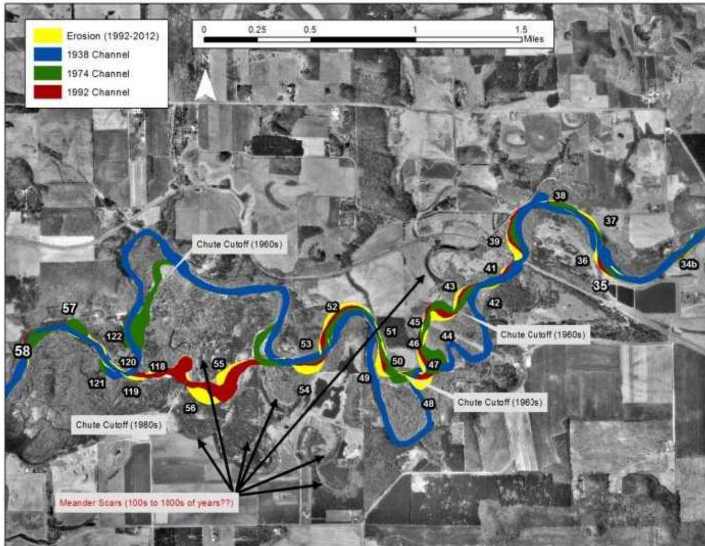
Figure 19. Erosion Sites along the focus reach, downstream of the Colfax wastewater treatment facility (1992-2012). This subreach has experienced multiple chute cutoffs since the 1960s, and relatively rapid channel adjustment along these sections since.
