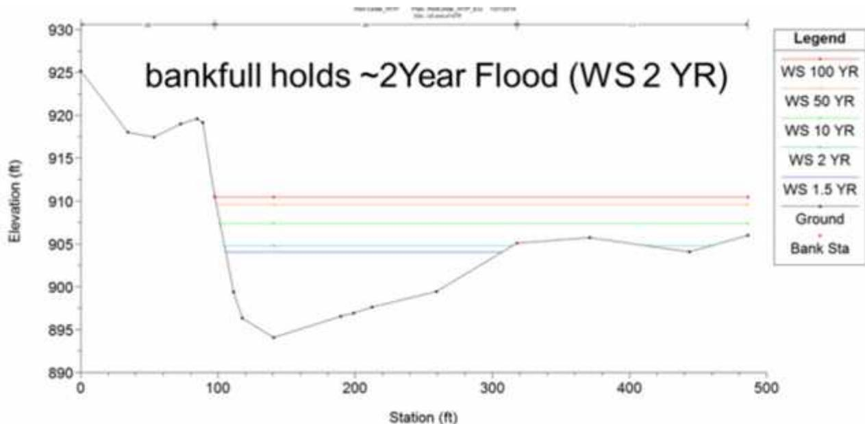
Figure 5. A cross section from the HEC RAS model at the upstream end of the wastewater treatment facility reach. Note that the channel bank tops (red dots) are reached during the 2-year flood. At the 100-year flood, less than 4 feet of water is on the floodplain.
