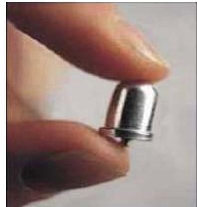
Figure 17 Mercury-containing auto switch
