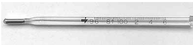
Figure 10 Mercury-containing fever thermometer
