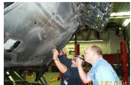
Figure 18 Checking for mercury-containing switches at WITC
