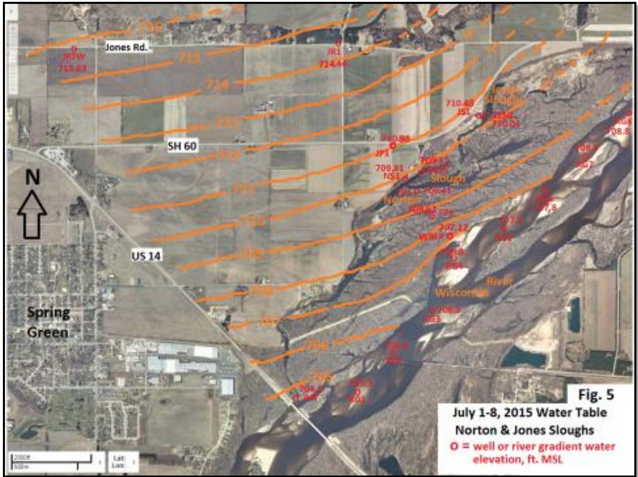
Figure 5: Groundwater flow map of the Norton and Jones Sloughs area
