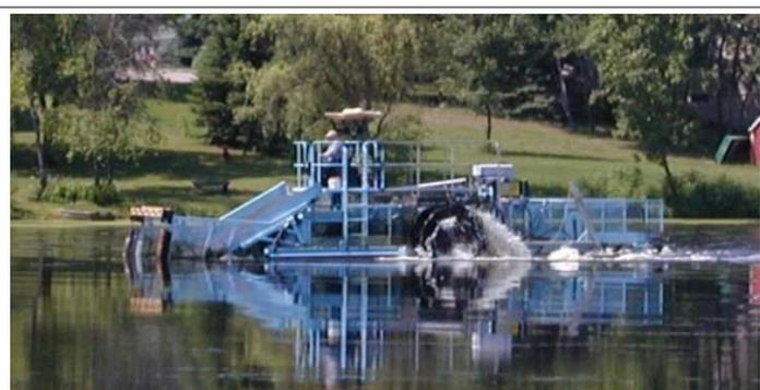
**Photograph 3.3-3. Mechanical harvester.**
